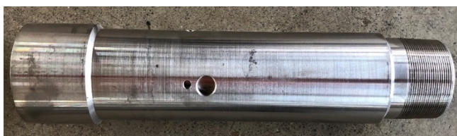
Fig 8. Physical diagram of pressure-drive pressure relief sliding sleeve
