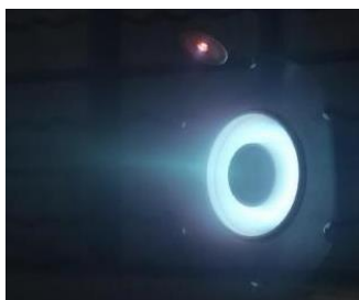
Figure 4. Low power Hall thruster operation with Xe at 200W-class
