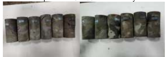
Figure 3-5: After the Brazilian splitting test of roof rock samples from 51206 return airway
