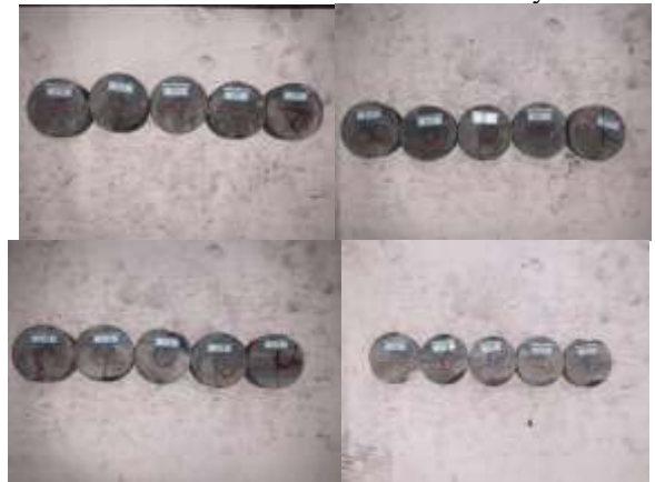
Figure 3-4: After the Brazilian splitting test of roof rock samples from 51207 return airway
