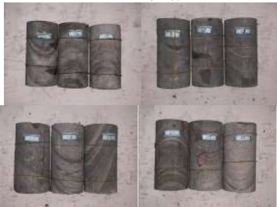
Figure 3-2: Results of Uniaxial compression failure test of roof rock samples from 51207 return airway
