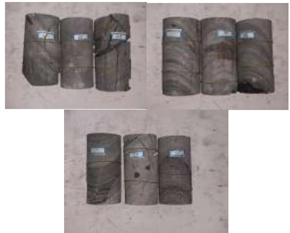
Figure 3-3: Roof rock samples after Uniaxial compression failure test from 51206 return airway
