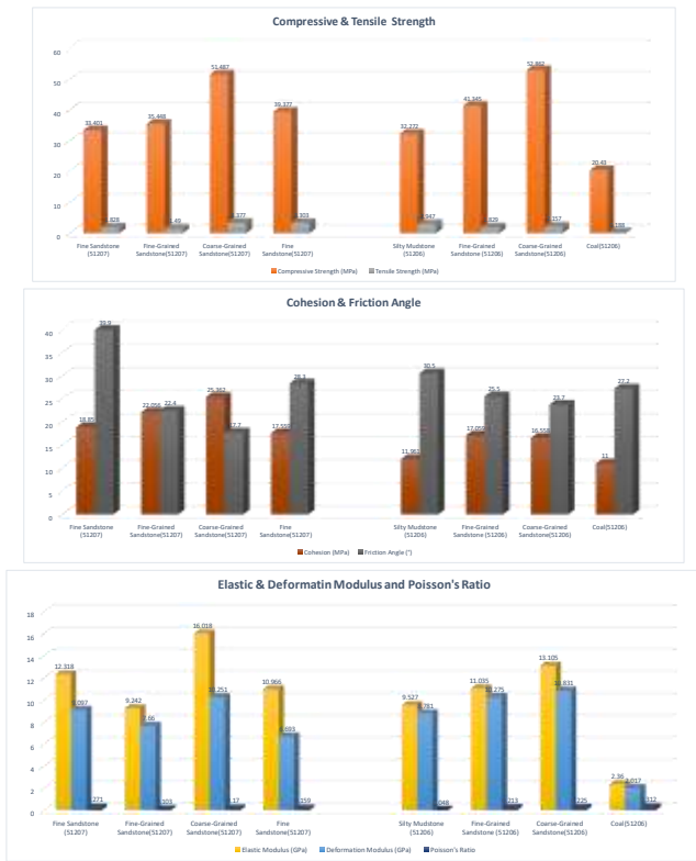
Figure 3-8: Mechanical Performance graph of roof rock samples from 51206 and 51207 return air roadway by lithology
