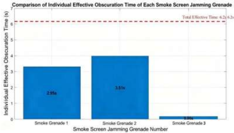
Figure 4 Comparison of individual effective shielding time of each smoke jamming bomb
