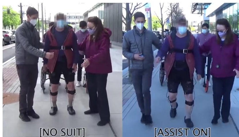
Figure 1. Using flexible wearable robots to help Parkinson's disease patients walk without freezing gait [14]
