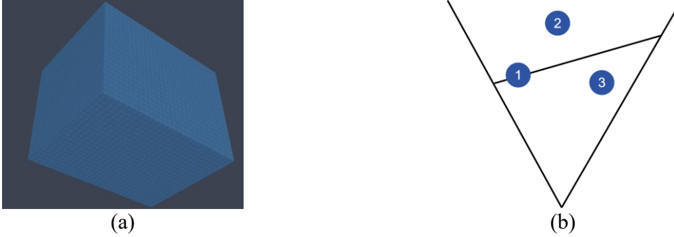
Figure 2. Figure (a) illustrates the view of an endoscope and a rectangular box of voxels. Figure (b) illustrates the sign of the SDF value. Voxel 1 represents an SDF value of near 0, voxel 2 shows an SDF value of smaller than 0, and voxel 3 has an SDF value bigger than 0.
