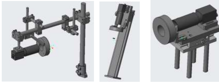
Figure 2 Outer CCD, top CCD, and inner CCD structures
